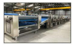
Gauge Roll Units engaged to reduce sheet thickness in progressive stages before cutting. The number of reduction stages may vary as per product or capacity requirements. Rotary Cutter to cut Dough blanks which prints excellent design on a continuously used Dough Sheet. The resulting network scrap Dough is set back to the scrap sheeter
